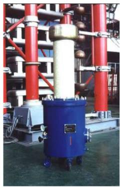
The transformers are designed for testing high voltage electrical equipment with power frequency voltage including tests at the site.
